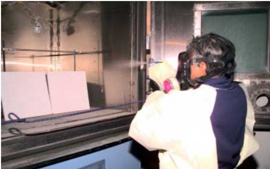
Figure 5-4. Application of BG Spores to Panels
